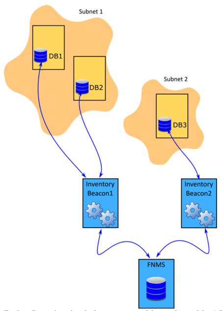
The above diagram shows three database servers, two on Subnet1 and one on Subnet2. The Subnet1 is assigned to Inventory Beacon1 and Subnet2 is assigned to Inventory Beacon2. Note that in this diagram, DB1 and DB2 are running versions of Oracle Database compatible with the same OLEDB driver, as discussed in Direct Collection of Oracle Inventory; separately, DB3 may also be compatible, or may require a different version, which may be the reason that it is managed by a separate inventory beacon.
