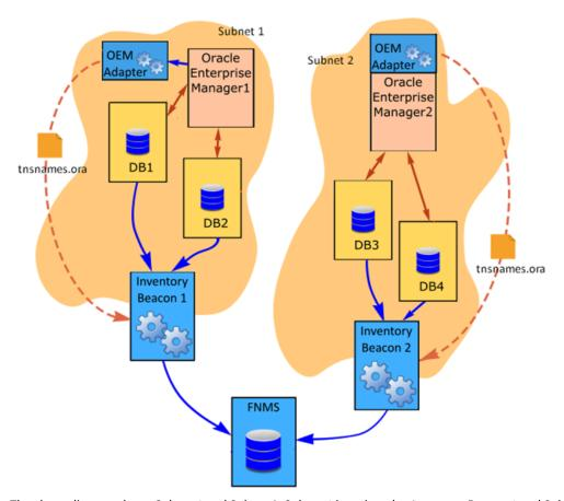
The above diagram shows Subnet 1 and Subnet 2. Subnet 1 is assigned to Inventory Beacon 1 and Subnet 2 is assigned to Inventory Beacon 2. Each subnet contains:
